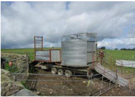
Mobile Sheep Dipper on 16ft Ifor Williams Tri axle Trailer with Honda WB20XT Pump and new pipes
