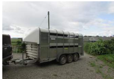
Mobile Sheep Dipper on 16ft Ifor Williams Tri axle Trailer with Honda WB20XT Pump and new pipes
