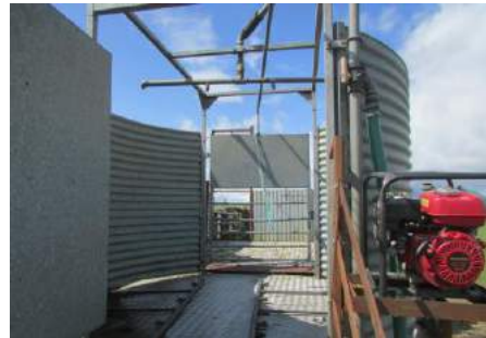
Mobile Sheep Dipper on 16ft Ifor Williams Tri axle Trailer with Honda WB20XT Pump and new pipes
